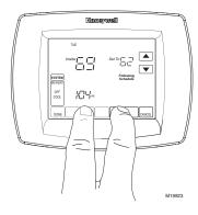
Fig. 16. Entering Installer Setup.
